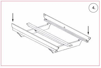
Insert the side panels with the spring into the groove of the angle sides and lightly thread the centrally seated fitting.
