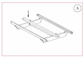
Place the support strip centrally on the foot sections and fix it to the foot sections with the 4 enclosed  $6 \times 80$  mm screws in accordance with point 5. The support strip is not needed for the 140 width.
