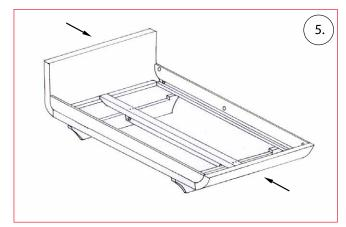
Attach the bed head and foot sections to the angle sides and side panels. Tighten the fitting in the centre of the side panel. Now screw the screws of the support strip to the foot sections.
