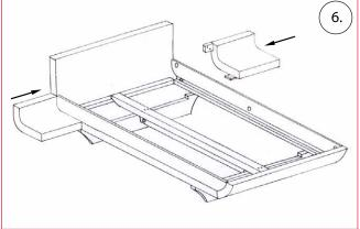
Fasten the console on the left and right in the cut-out on the back of the headboard and the underside of the angle sides, using two 4 × 35 mm screws apiece.
