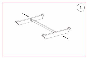
Screw the crossbar together with the 2 foot sections. There are 2 crossbars for the 140 width.
