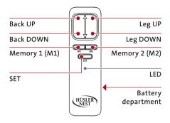
Operate back- and leg up position synchronously: Operate buttons «back» and «leg» simultaneously
