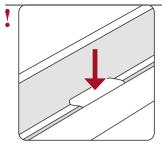
All six support points of the insert frame must be situated in the correct position (sidebars/ centre beam)
