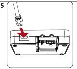
Connect power cable to the control box and then to the power system (supply voltage and input voltage on the type plate must be identical)
