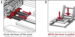
Draw red lever of the zone which is to be lowered into the direction of the middle of the bed
