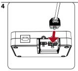
Connect control box to motor
