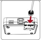
Connect control box to motor
