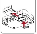
Put two new batteries type AAA (no rechargeable ones) into the control box, watch out for correct polarity! If the control box peeps, the battery voltage is too low > replace batteries
