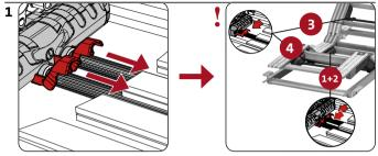
Draw red lever of the zone which is to be lowered into the direction of the middle of the bed
