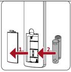
Put two new batteries type AAA (no rechargeable ones) into the remote control, watch out for correct polarity! 3
