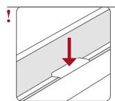
All six support points of the insert frame must be situated in the correct position (sidebars/centre beam)
