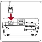
Connect power cable to the control box and then to the power system (supply voltage and input voltage on the type plate must be identical)
